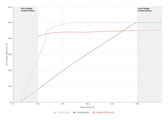
The recommended RPM range for this motor is 360-1800 RPM. Operating below 360 RPM is not advised except during coasting or ramp-up. For operation outside of this recommended range, please contact Infinitum for a customized solution. These curves are for reference only; actual performance may vary.
