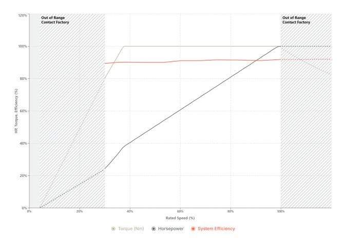
The recommended RPM range for this motor is 720-2400 RPM. Operating below 720 RPM is not advised except during coasting or ramp-up. For operation outside of this recommended range, please contact Infinitum for a customized solution. These curves are for reference only; actual performance may vary.
