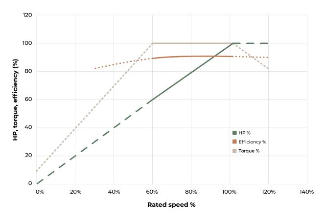
Note: Infinitum does not recommend using the motor below 60% of rated speed at full torque except when coasting or ramping up. It is also essential to restrict power and FLA within the nameplate rating when operating the motor above 100% of its rated speed. To operate the motor outside the recommended operating range, please contact the factory and our Application Engineers will provide a customized solution.
