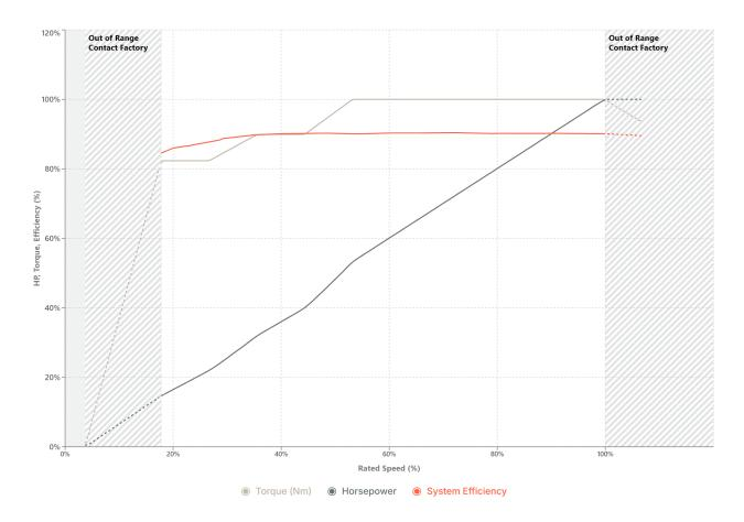
The recommended RPM range for this motor is 480-2700 RPM. Operating below 480 RPM is not advised except during coasting or ramp-up. For operation outside of this recommended range, please contact Infinitum for a customized solution. These curves are for reference only; actual performance may vary.
