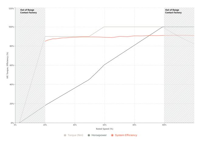
The recommended RPM range for this motor is 720-3600 RPM. Operating below 720 RPM is not advised except during coasting or ramp-up. For operation outside of this recommended range, please contact Infinitum for a customized solution. These curves are for reference only; actual performance may vary.
