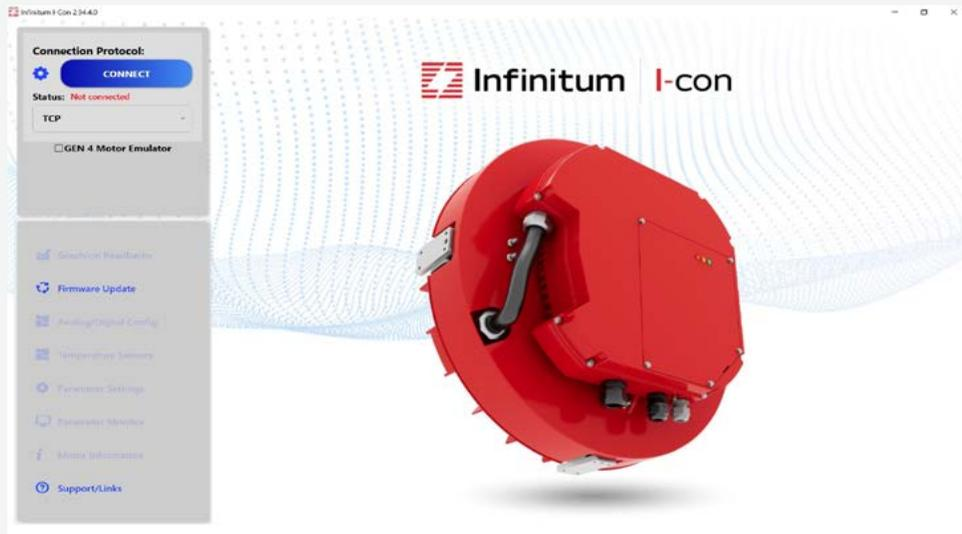
Once the motor is connected to the computer, the “Status” in the upper left box should indicate “Connected” in green text and the connect button changes to a red “DISCONNECT” button as indicated in Figure 5. This button is used to break the connection between I-con and the motor.
