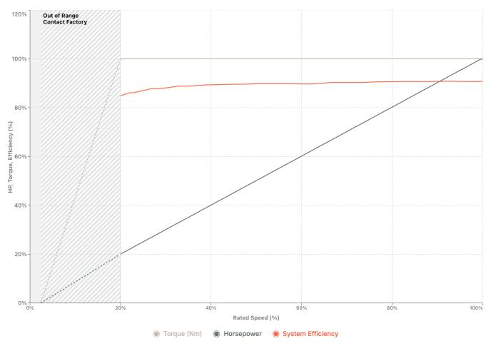
The recommended RPM range for this motor is 840-4200 RPM. Operating below 840 RPM is not advised except during coasting or ramp-up. For operation outside of this recommended range, please contact Infinitum for a customized solution. These curves are for reference only; actual performance may vary.
