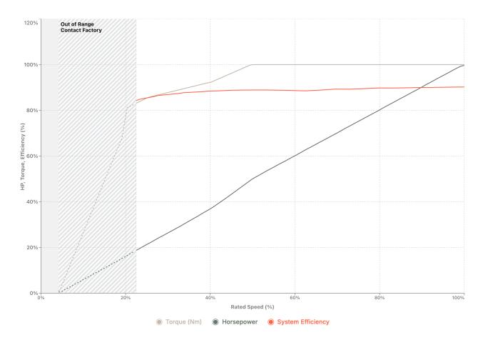
The recommended RPM range for this motor is 540-2400 RPM. Operating below 540 RPM is not advised except during coasting or ramp-up. For operation outside of this recommended range, please contact Infinitum for a customized solution. These curves are for reference only; actual performance may vary.
