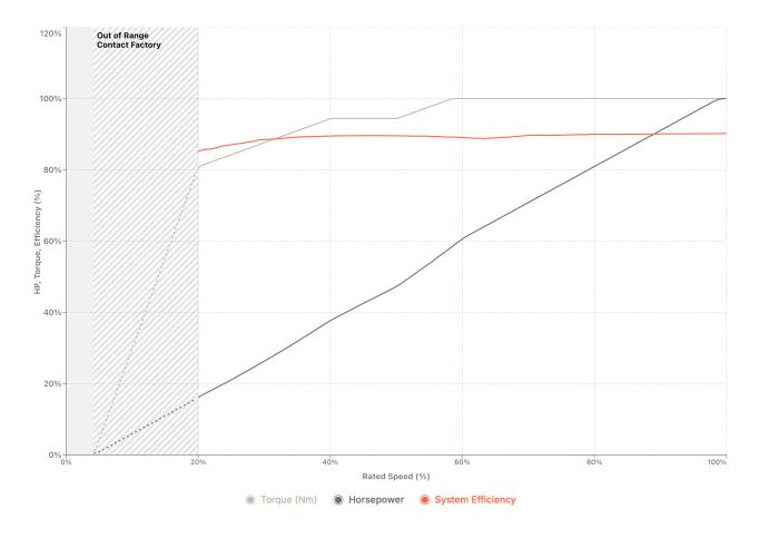
The recommended RPM range for this motor is 480-2400 RPM. Operating below 480 RPM is not advised except during coasting or ramp-up. For operation outside of this recommended range, please contact Infinitum for a customized solution. These curves are for reference only; actual performance may vary.
